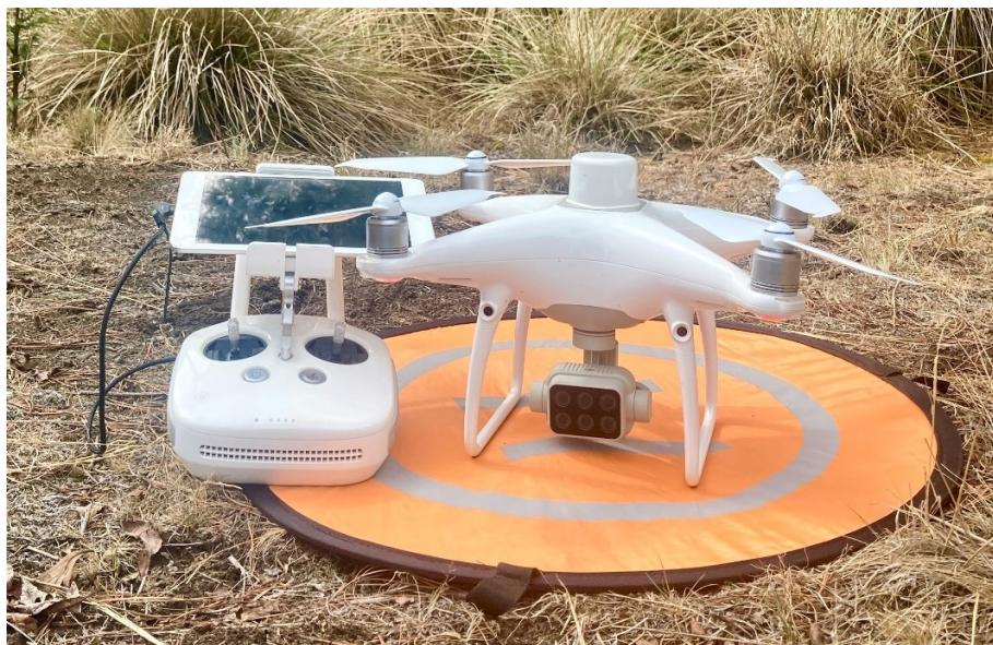
**Figure 2.** DJI Phantom 4 Multispectral quadcopter used to acquire images, together with the remote control and mobile device (iPad) used to visualize the Ground Station Pro flight application.
