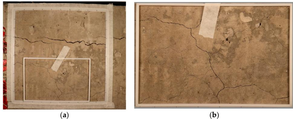
**Figure 5.** (a) A perspective frame affixed at the lower part of the reference frame and (b) the perspective frame in the full field of view after zooming in.
