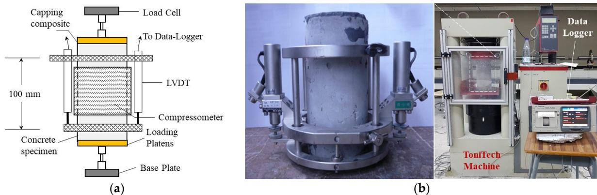
**Figure 9.** The uniaxial compression test: (a) representatives chart and (b) testing system.
