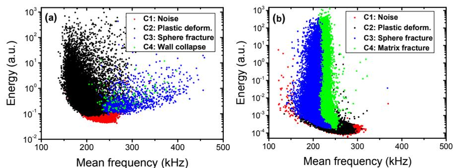
**Figure 3.** The 2D projection of the clusters to the energy-mean frequency space for (a) Al foam; (b) AlSi12 foam.
