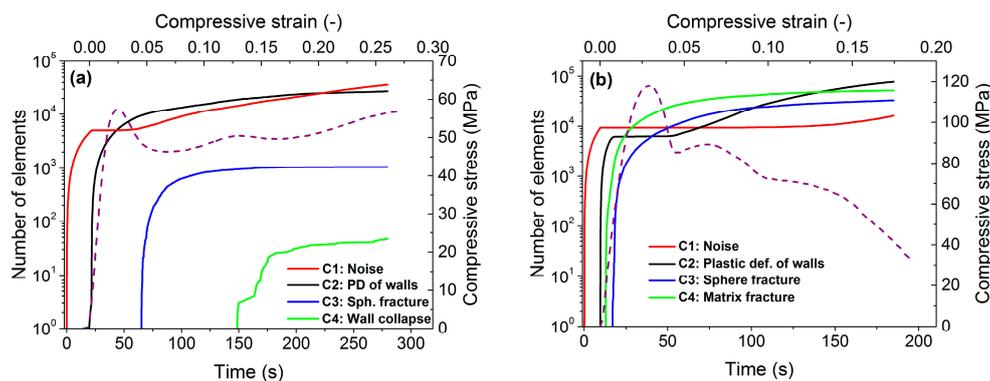
**Figure 2.** Time evolution of the cumulative number of elements in different AE clusters in (a) Al foam; (b) AlSi12 foam. Red line—noise; black—plastic deformation of matrix; blue—sphere fracture; green—Cluster 4: wall collapse in Al foam and brittle phase fracture of the matrix in AlSi12 foam. The stress-strain curve (dashed line) is also displayed.
