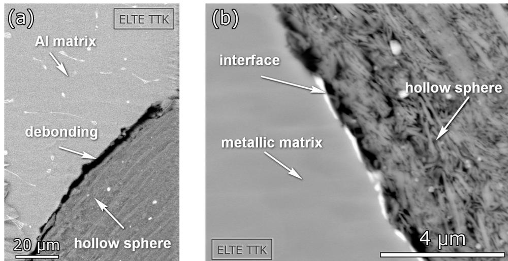
**Figure 5.** SEM micrographs showing (a) debonding of ceramic spheres from the Al matrix and (b) layered structure of the ceramic spheres.
