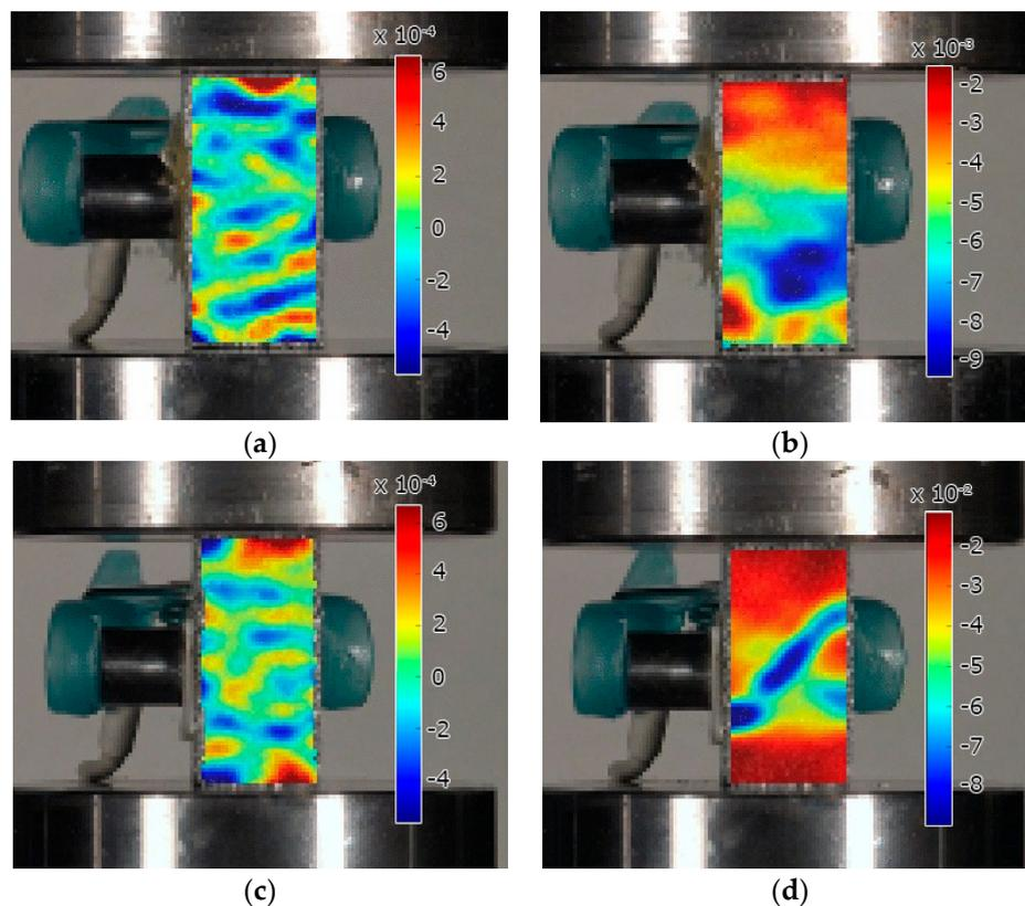
**Figure 7.** Surface  $\epsilon_{yy}$  strain maps at different macroscopic strain: (a) Al foam at 2%; (b) Al foam at 4%; (c) AlSi12 foam at 2%; (d) AlSi12 foam at 4%. (The scale of  $\epsilon_{yy}$  strain is different in each figure.).
