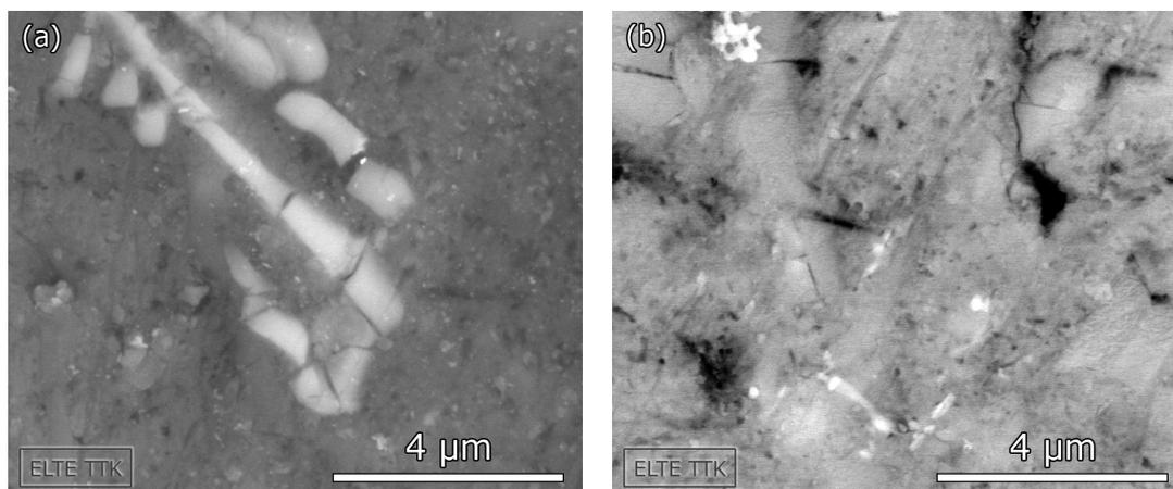
**Figure 6.** SEM images of the fractured brittle phases (a) Al-Si-Fe intermetallic phase; (b) Si phase.
