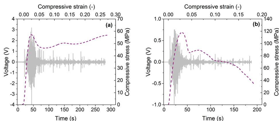
**Figure 1.** Typical compressive stress-strain curves (dashed line) and acoustic emission (AE) signals (grey line) for metal matrix syntactic (MMS) foams with (a) Al matrix; (b) AlSi12 matrix.
