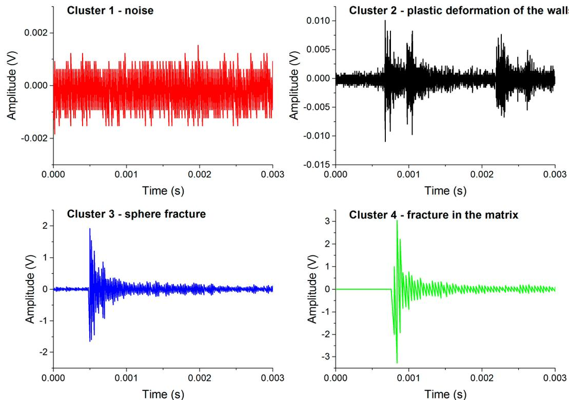
**Figure 4.** Characteristic AE waveforms corresponding to different clusters in AlSi12 foam: Cluster 1: noise; Cluster 2: plastic deformation of the walls; Cluster 3: sphere fracture; and Cluster 4: fracture in the brittle phase of the matrix.
