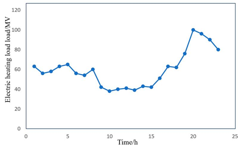
**Figure 6.** Daily load curve of a power supply and distribution system.
