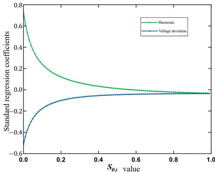
Figure 4. The regression coefficients of PQ cost with the primary evaluation indicators in the first layer.
