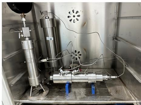
**Figure 2.** The core gripper used in the experiment.
