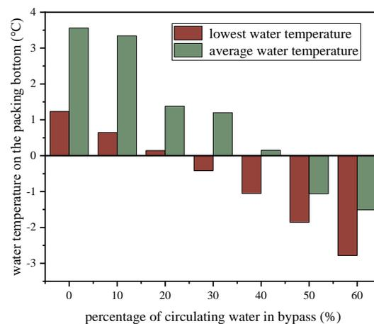
**Figure 8.** Effect of water bypass percentage on the lowest and average water temperatures on the packing bottom.
