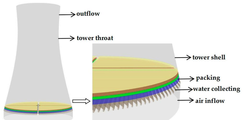
**Figure 1.** Schematic of High-Level Wet Cooling Tower.
