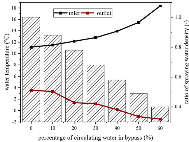
**Figure 5.** Effect of the water bypass percentage on the inlet and outlet temperatures and the spray density.
