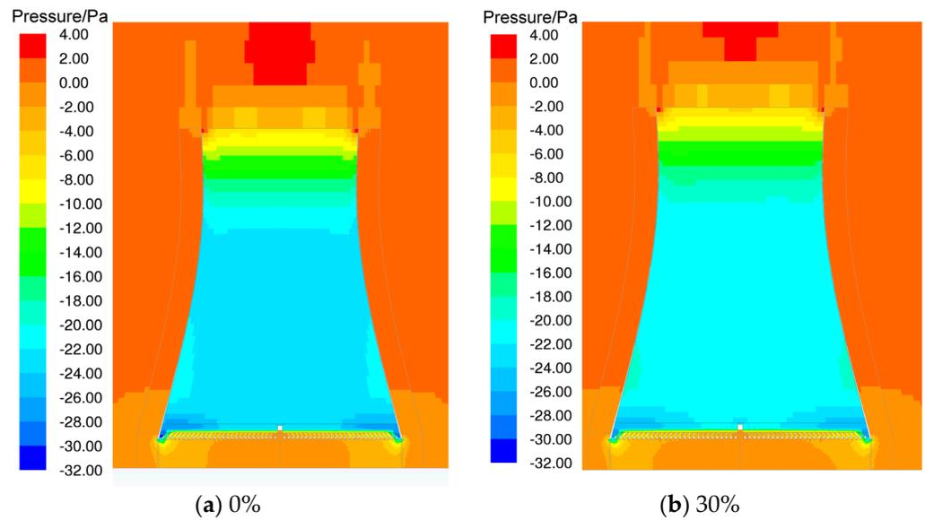
**Figure 7.** Cooling tower profile pressure distribution for different bypass water percentages, (a): 0%, (b): 30%.
