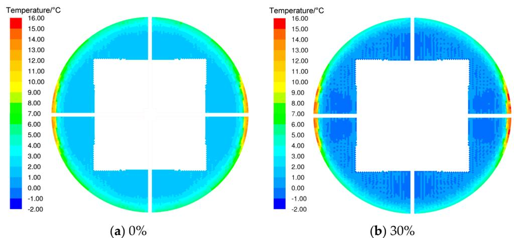
**Figure 6.** Distribution of the water temperature at the bottom of the packing at different bypass water percentages, (a): 0%, (b): 30%.
