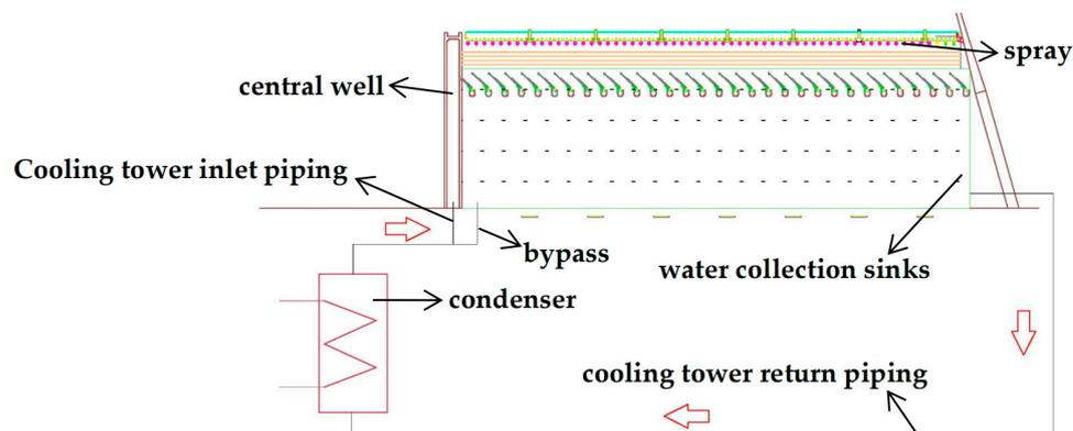
**Figure 4.** Schematic illustration of the circulating water bypass design.
