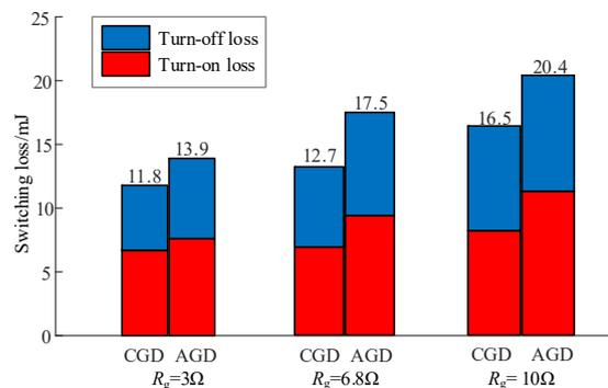
Figure 11. Switching loss at different gate resistances.
