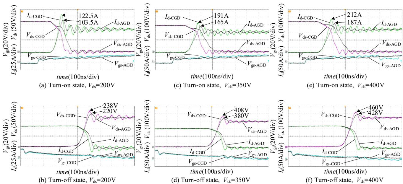
**Figure 9.** Turn-on and turn-off waveforms at different values of  $V_{ds}$ .
