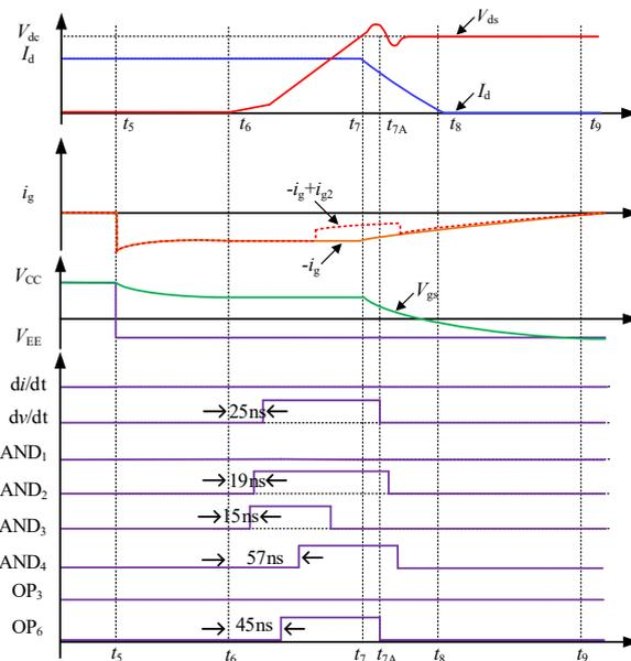
Figure 6. The turn-off characteristics of AGD.
