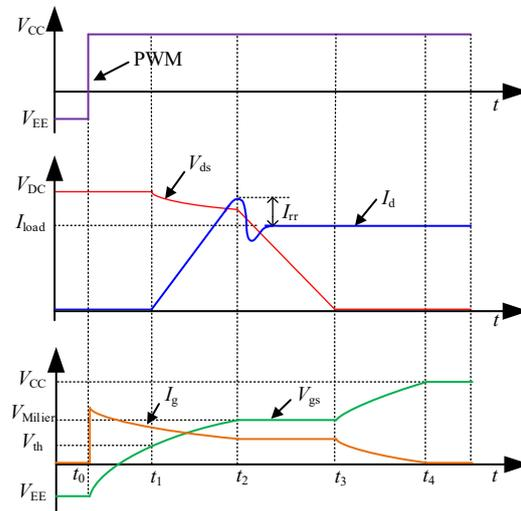
**Figure 2.** The turn-on characteristics of SiC MOSFET.
