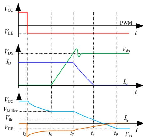
Figure 3. The turn-off characteristics of SiC MOSFET.
