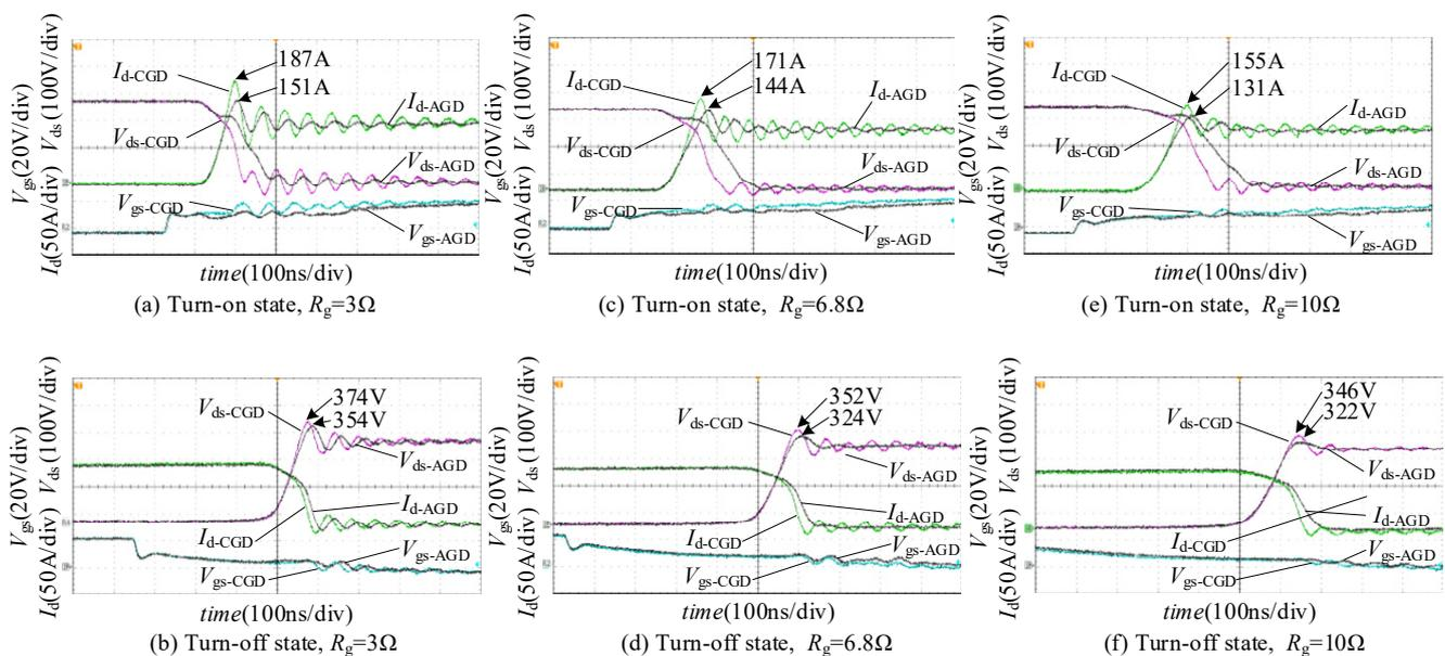
**Figure 8.** Experimental waveforms of AGD and CGD under different values of  $R_g$ .
