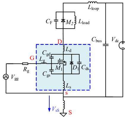
**Figure 1.** Equivalent circuit model for the double-pulse test configuration.
