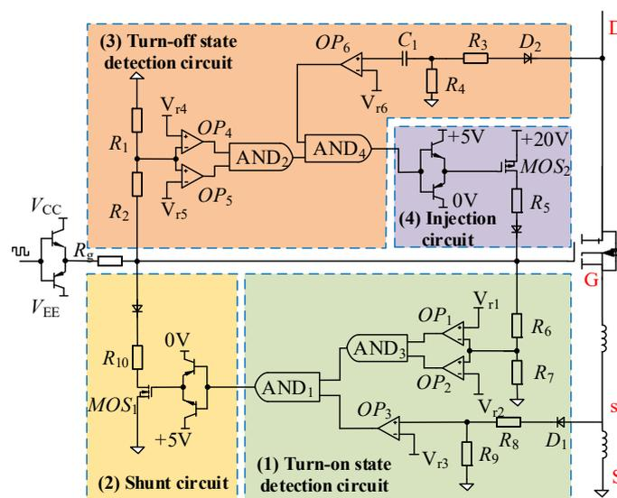
Figure 4. Schematic of the proposed AGD.
