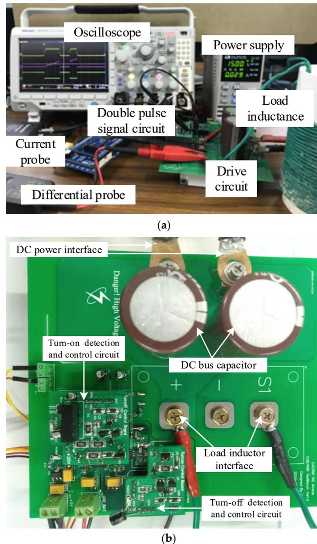
**Figure 7.** The double-pulse testing experimental platform and circuit. (a) Experimental platform; (b) proposed active gate drive circuit.
