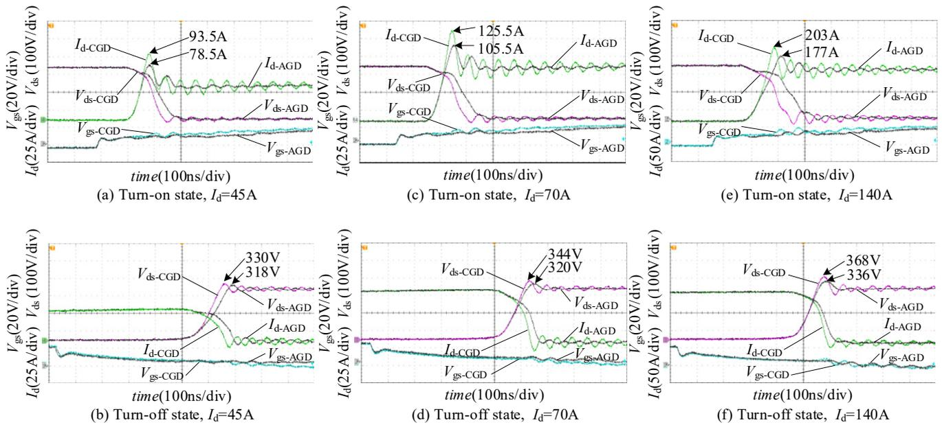
Figure 10. Turn-on and turn-off waveforms at different values of  $I_d$ .
