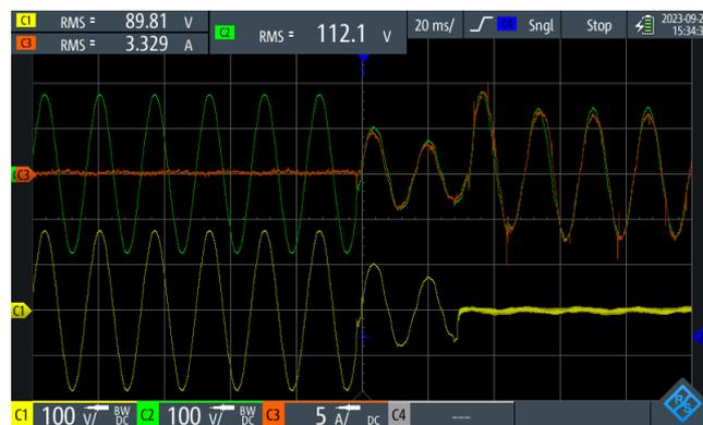
Figure 30. Islanding procedure during the loss of main grid.
