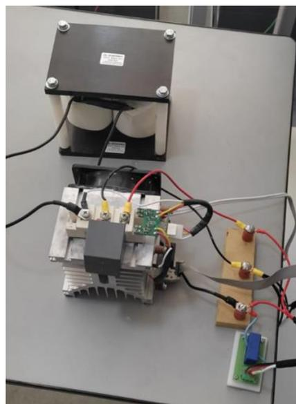
**Figure 13.** DC-DC boost converter.
