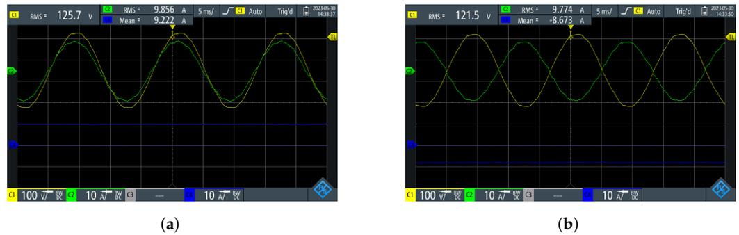
Figure 26. Converter operating modes: (a) injection mode; (b) absorption mode.
