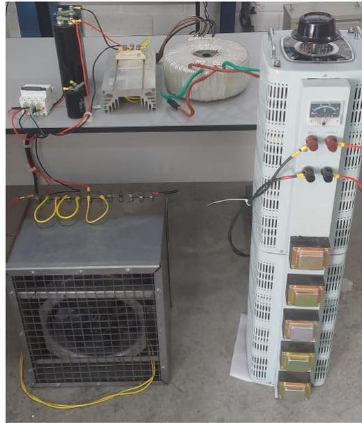
Figure 8. TEG system emulator circuit.
