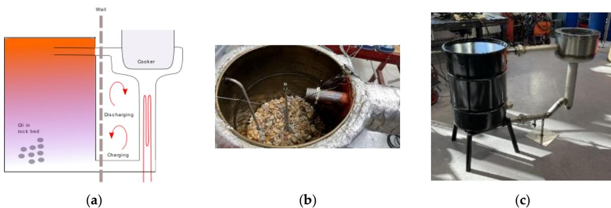
**Figure 22.** Single-tank heat storage system with external cooker. (a) Concept diagram; (b) Rock bed before thermal oil is inserted; (c) Prototype (without insulation).
