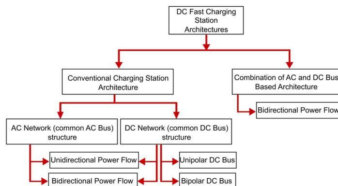
**Figure 6.** The classification of DC fast-charging station architectures.
