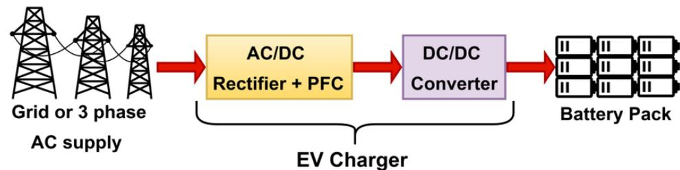
**Figure 2.** The basic concept of an EV charger.
