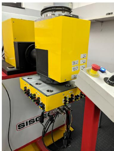
**Figure 7.** Calibration bench for the inclinometer sensors.
