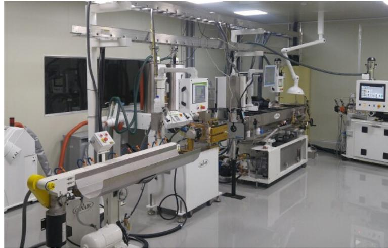
**Figure 1.** Medical multi-lumen tubing extrusion system.
