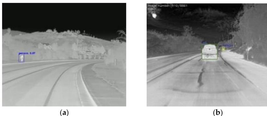
**Figure 6.** FLIR ADAS thermal image for walking people and cars on the road (a) people walking on the road marked with blue box, (b) Car driving on the road with green box. Teledyne FLIR LLC (2022) [22].
