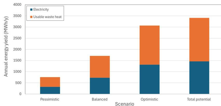
**Figure 8.** Analysis of annual energy yield in terms of electricity and usable waste heat from biodegradable municipal waste and livestock manure using anaerobic digestion and combustion of the biogas in an internal combustion engine.
