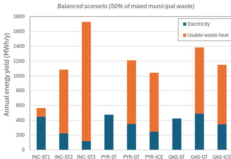
**Figure 6.** Analysis of annual energy yield in terms of electricity and usable waste heat from mixed municipal waste using nine different thermochemical processes. Data are shown for the balanced scenario.
