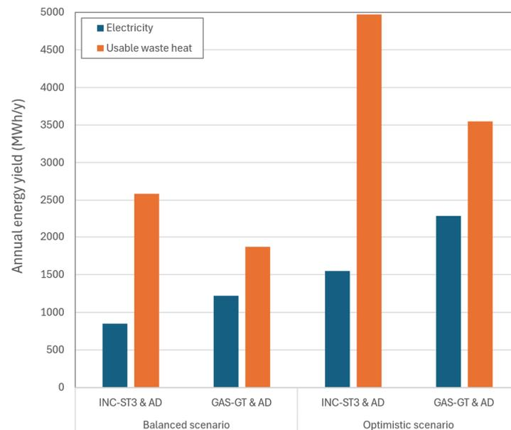
**Figure 10.** Analysis of annual energy yield in terms of electricity and usable waste heat utilizing all waste sources and combining two thermochemical processes with anaerobic digestion. Data are shown for the balanced and the optimistic scenario.
