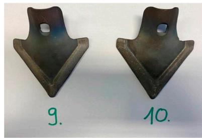
**Figure 6.** The samples made through laser cladding (source: self-made).
