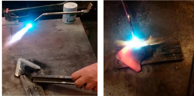
**Figure 4.** Application of a layer via hot metal powder spraying (source: self-made).
