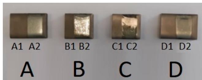
**Figure 7.** Samples remelted with a flame on the left and with a laser on the right (source: self-made).
