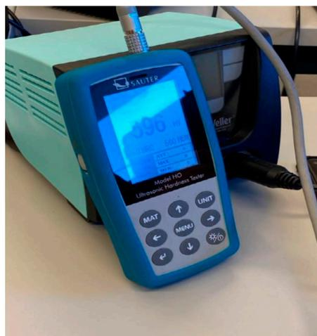
**Figure 8.** SAUTER HO ultrasonic hardness tester (source: self-made).
