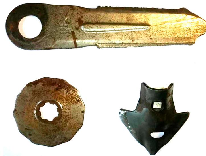
**Figure 1.** Worn agricultural machine parts. Corn-stalk crushing knives; disc of corncob breaking adapter; cultivator tine [16].
