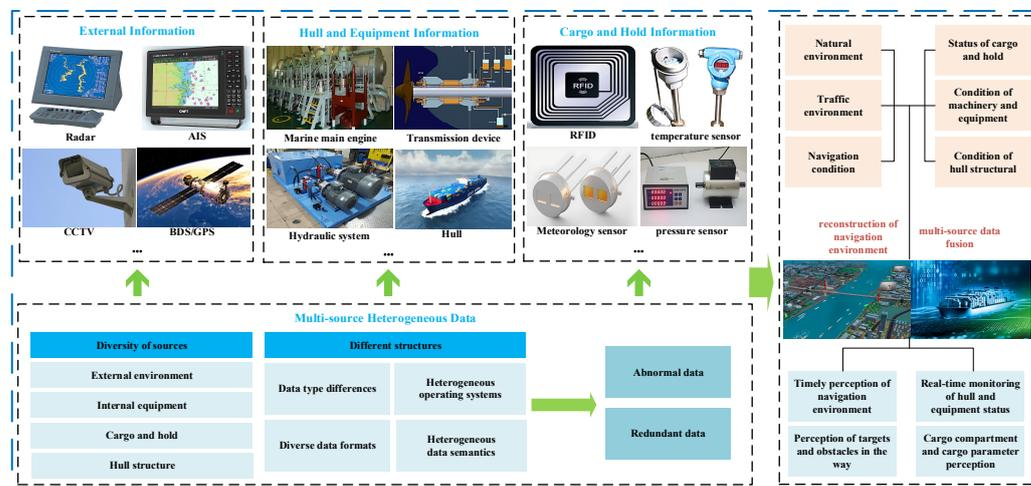
Figure 2. Ship intelligent perception technology diagram.
