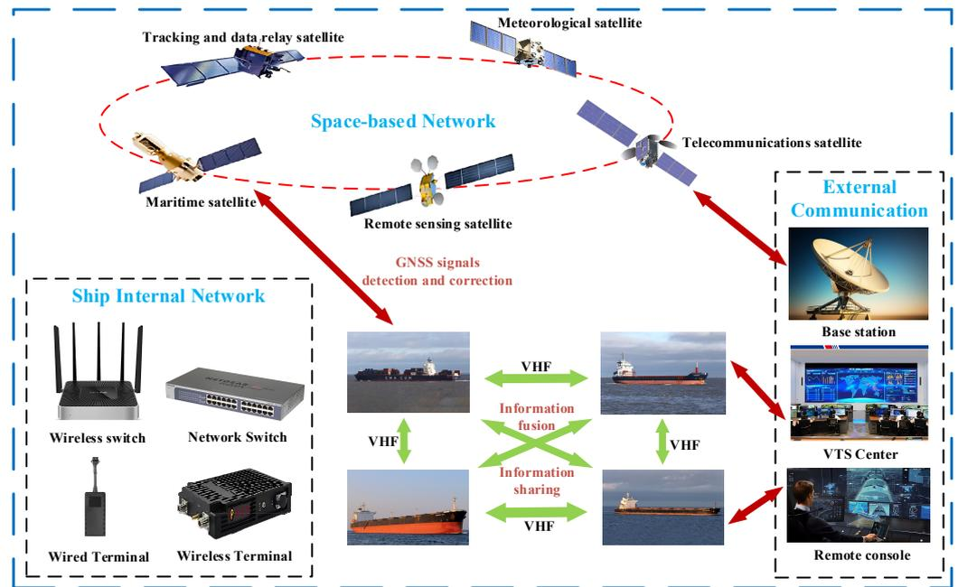
Figure 3. Ship intelligent communication technology diagram.
