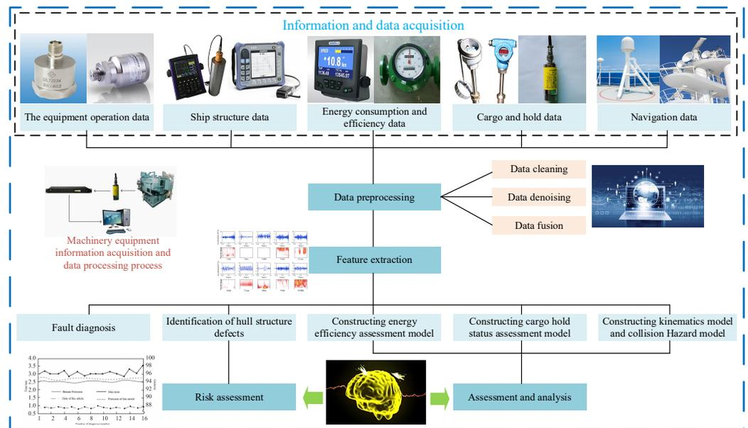
Figure 4. Ship intelligent assessment technology diagram.
