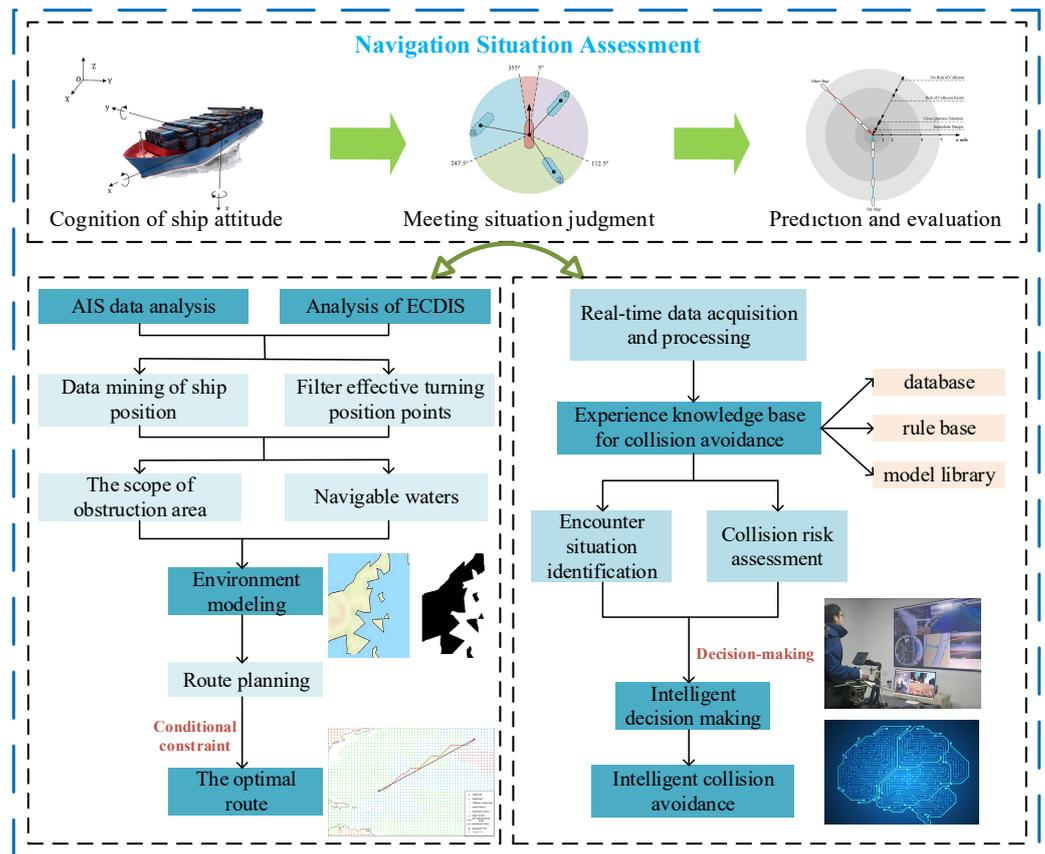
Figure 5. Ship intelligent decision-making technology diagram.
