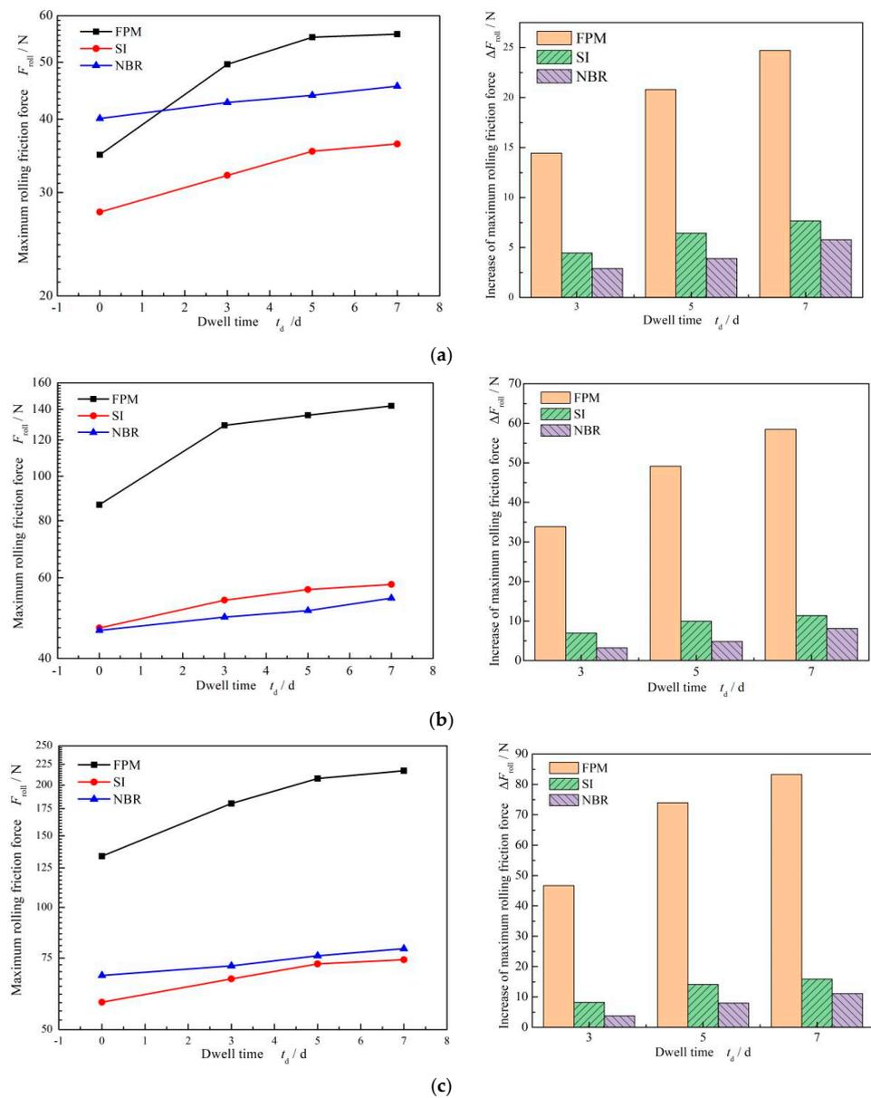
**Figure 13.** Influence of dwell time on the rolling friction force of different O-ring materials: (a)  $\epsilon = 9\%$ . (b)  $\epsilon = 12\%$  and (c)  $\epsilon = 12\%$ .
