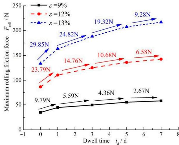
Figure 7. The effect of different compression ratios on the static friction force of FPM O-rings.
