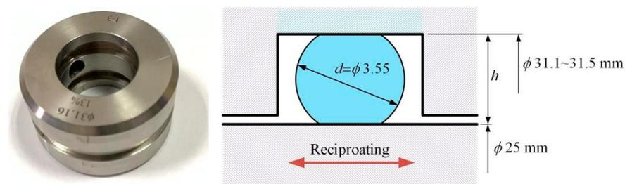
**Figure 3.** Diagram of O-ring compression installation.
