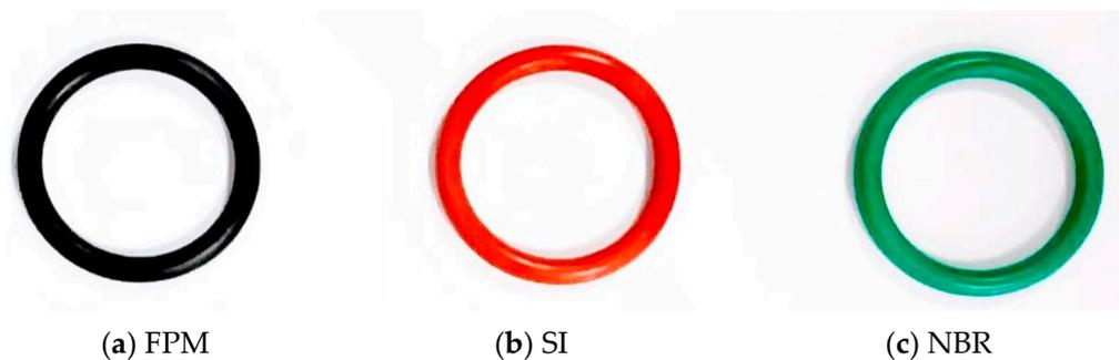
**Figure 2.** Rubber O-ring samples.
