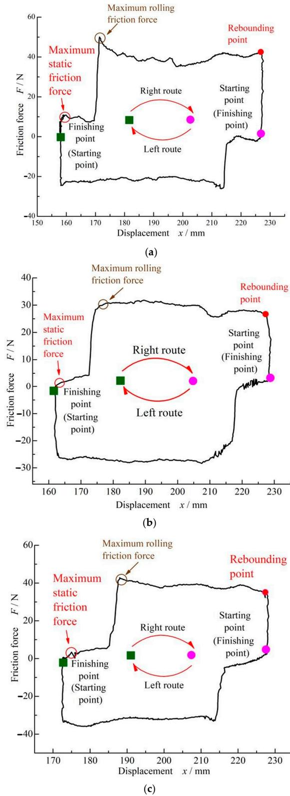
**Figure 12.** Reciprocating cycle curves of different O-ring material at  $\epsilon = 9\%$  and  $p = 0$  after a 3-day dwell period: (a) FPM O-ring. (b) SI O-ring. (c) NBR O-ring.
