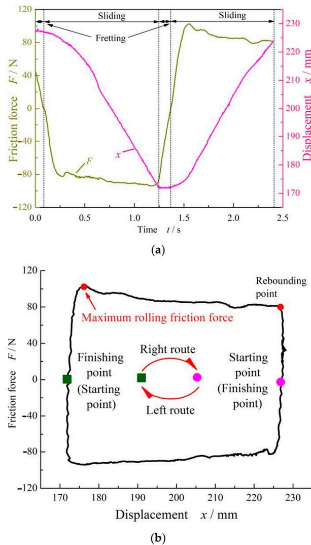
**Figure 9.** Reciprocating cycle curve of FPM O-rings at  $\varepsilon = 9\%$  and  $p = 0.5$  MPa without dwell periods: (a) friction and displacement time-varying curves. (b) Friction–displacement curve.
