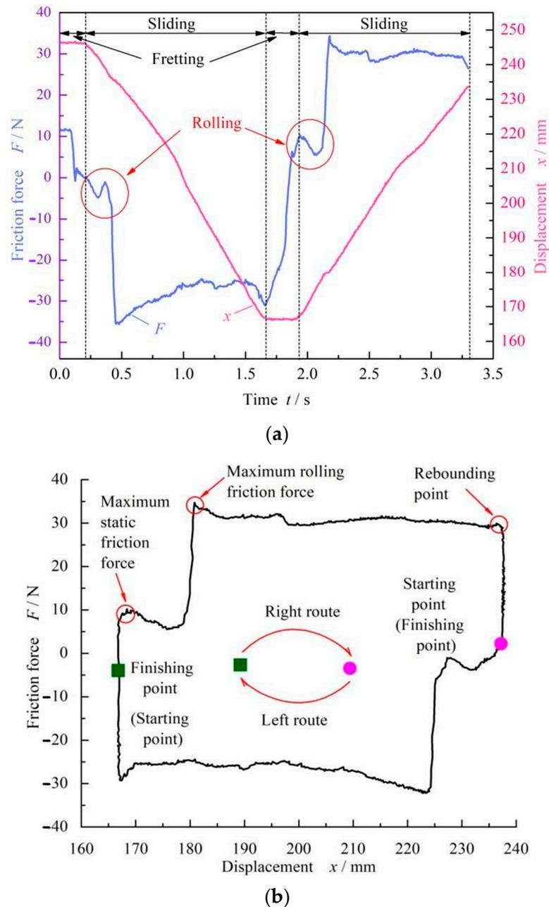
**Figure 4.** Reciprocating cycle curve of FPM O-rings at  $\varepsilon = 9\%$  and  $p = 0$  MPa without dwell time: (a) friction force and displacement time-varying curves and (b) friction force–displacement curve.
