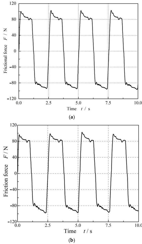
**Figure 10.** Reciprocating cycle curve of FPM O-rings at  $\epsilon = 9\%$  and  $p = 0.5$  MPa: (a) without dwell and (b) 1-day dwell.
