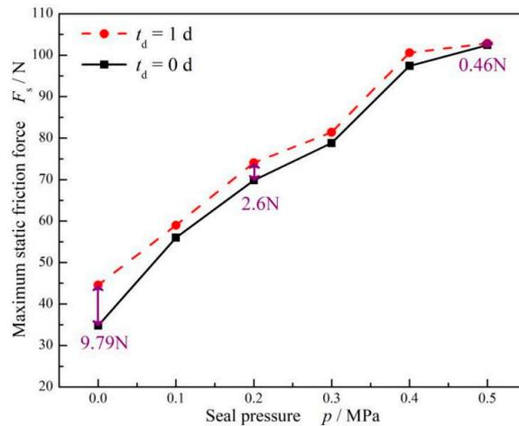
**Figure 11.** Influence of seal pressure on the maximum static friction force ( $\epsilon = 9\%$ ).
