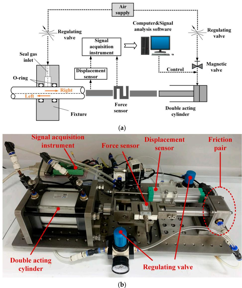
**Figure 1.** O-ring reciprocating motion test device: (a) principal diagram of the experimental device and (b) physical experimental device diagram.
