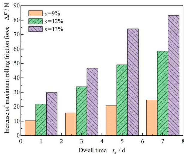
Figure 8. Influence of dwell time on the increase in the maximum static friction force of FPM O-rings under different compression settings.
